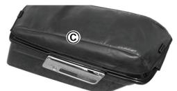
Each Saddlebag Chap will have six mounting tabs; pull each tab through to the underside of the lid and mark the lid with some reference points (D). Smooth out and pull the cover snug as you do this so the tabs will best be in their final position.
