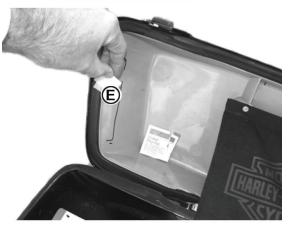
NOTE: One side of the hook-n-loop fastener tape is sewn to the Saddlebag Chap. The other side has an adhesive backing with protective paper. Remove the hook fastener strips from the chap's mounting tabs. Then remove the backing tape from each hook fastener strip and press it into place on the inside of the saddlebag lid (F).
